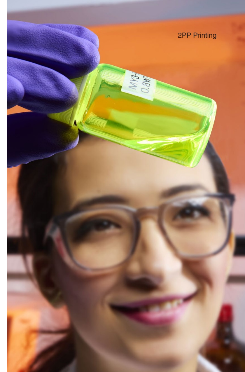
Research scientist Magi Yassa holds a sample of the team’s dual-wavelength photo resin. The liquid monomer resin is being developed to solidify, or “cure,” in different ways when it absorbs different colors of light, enabling researchers to print both solid and porous features using the same material.
