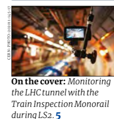
On the cover: Monitoring the LHC tunnel with the Train Inspection Monorail during LS2. 5
