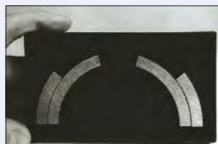
A model of the cross-section of the new niobium-tin superconducting dipole magnets, showing the two-layer structure of the coil.
